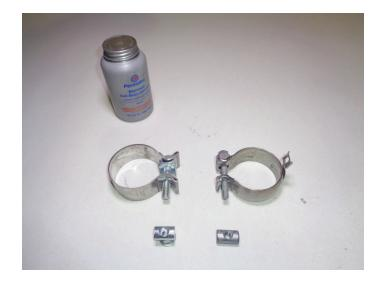
8. Place clamp (MC250BS) on muffler (71416-533) outlet. Fasten muffler onto catalytic converter using (x2 ea.) flat washers (HW303) and hex nuts (HW106).
