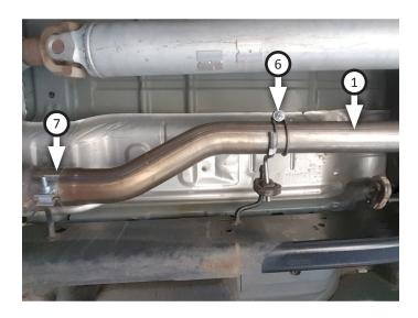
10. Place **clamp hanger (5)** onto **muffler (2)** then connect it to inlet pipe, inserting wire hanger into factory isolator. Tighten clamp hanger just enough to allow for adjustment. Place **clamp (7)** onto muffler outlet.
