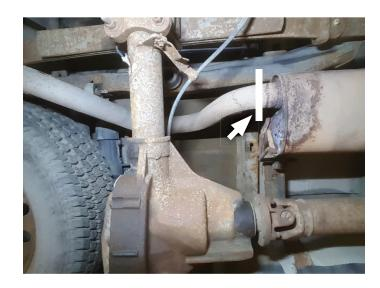
4. Remove band clamp securing factory inlet pipe to converter Y-Pipe. Dismount wire hangers from mounts then remove muffler assembly and set aside.
