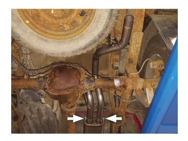
13. Secure **rear frame mount (12)** to vehicle using **bolt (14)** through frame, mount, **flat washer (16)**, **lock washer (17)** and **nut (15)**. Fit **rubber hanger (13)** onto mount.
