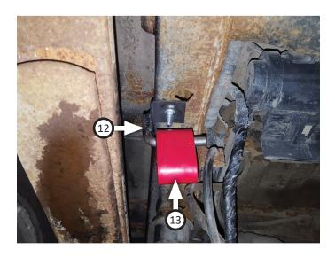
14. Place clamp (11) onto left rear tailpipe (6) then connect it to left front tailpipe. Insert wire hanger into rubber hanger then tighten clamp just enough to allow for adjustment.
