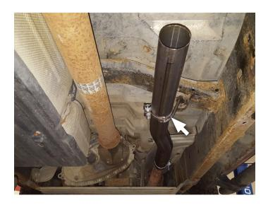
11. Place clamp (10) onto muffler (2) inlet then connect muffler to inlet pipe or extension. Tighten clamp just enough to allow for adjustment. Place (x2) clamps (11) onto muffler outlets.
