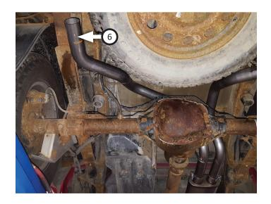
15. Place (x2 ea.) clamps (11) onto side exit pipes (7) then connect them to tailpipes. Tighten clamps just enough to allow for adjustment.
