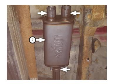
12. Route **right (5)** and **left front (4) tailpipe** over axle and connect them to muffler outlets. Insert wire hangers into isolators then tighten clamps (x2) just enough to allow for adjustment.
