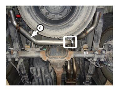
16. Place (x2 ea.) clamps (12) onto side exit pipes (7) then connect them to rear tailpipes. Tighten clamps just enough to allow for adjustment.
