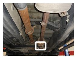
4. Disconnect factory muffler wire hangers (x2) from isolators on vehicle frame.
