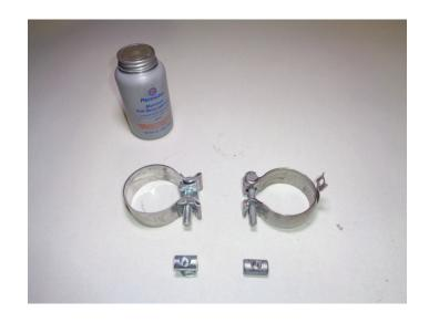
www.flowmastermufflers.com Technical Support (866) 464-6553 7. Place ball clamp (removed step 4) onto **inlet pipe (1)** then connect it to catalytic converter. Insert wire hanger into isolator and tighten clamp just enough to allow for later adjustment. **NOTE:** For some early 2009 models, the mount hanger is attached further rearward on frame. In this case, install **front clamp hanger (6)** onto inlet pipe then insert it into isolator.
