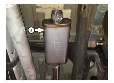
Route tailpipe assembly (4) over axle and connect it to muffler outlet. Mount wire hangers into isolators (x3) then tighten clamp enough to allow for adjustment.
