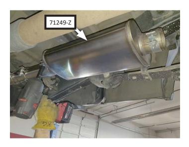
Route tailpipe assembly (26754M) over axle and connect it to muffler outlet. Mount wire hangers into isolators (x2) then tighten clamp enough to allow for adjustment.
