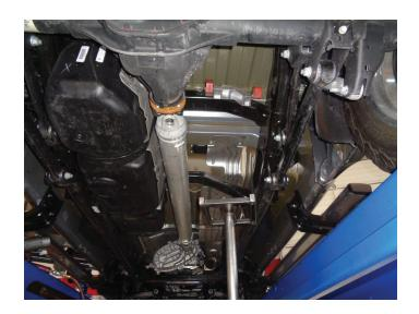
7. Remove stock studs from catalytic converter flange.
