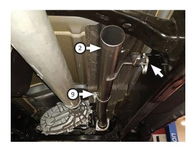
12. Place clamp (9) onto muffler (3) inlet, then connect muffler to extension. Tighten clamp on muffler inlet just enough to allow for adjustment. Place (x2) clamps (10) onto muffler outlets.
