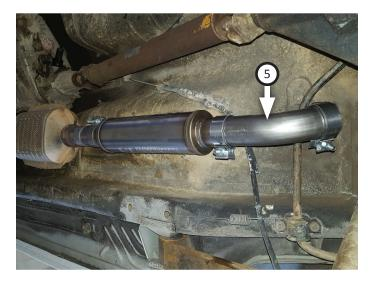
11. Route **tailpipe assembly (6)** over axle and connect it to front tailpipe. Insert wire hangers (x2) into isolators and tighten clamp enough to allow for adjustment.
