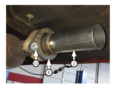
8. Place **clamp (10)** onto **FFX muffler (4)** then connect it to inlet pipe. Tighten clamp just enough to allow for adjustment. Set another **clamp (10)** onto muffler outlet.
