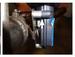
**NOTE:** Offset outlet pipe should be oriented to passenger side during install.
