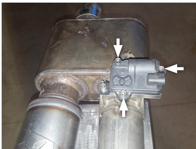
9. Install muffler into cut out section of factory exhaust then secure it using (x2) **clamps (8)**. Tighten them just enough to allow for adjustment.
