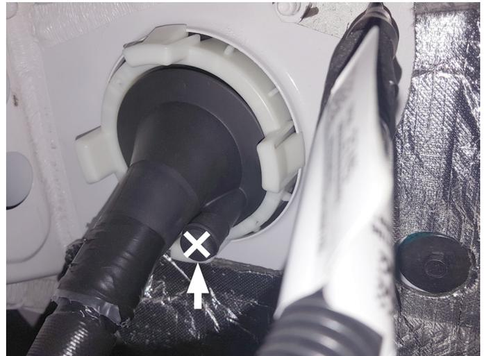
16. Thread hanger wire into cab through firewall, then bend its end and connect it to controller kit. Tape over connection to secure it.
