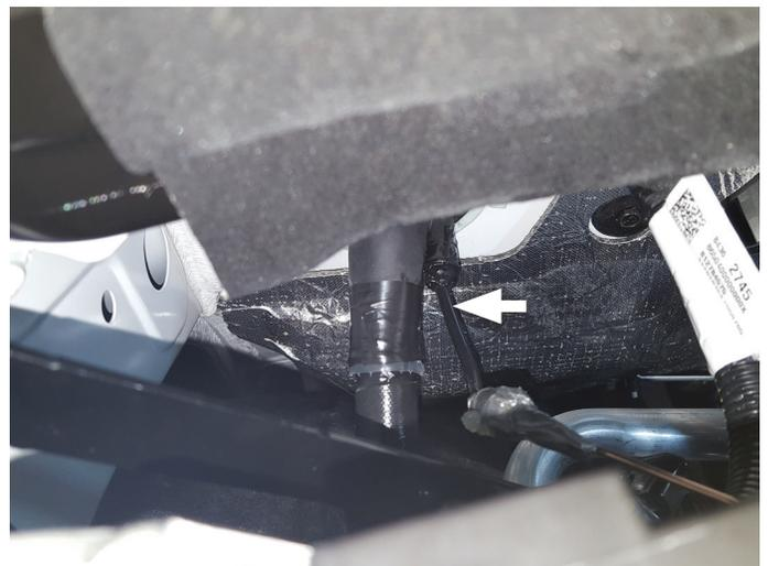
18. Fasten controller kit to a point up and away from interfering with passengers feet.
