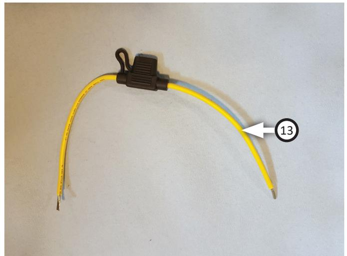
13. Cut off connector on end of **controller kit (5)** red wire. Place **butt connector (16)** onto inline fuse holder then attach it to red wire. Crimp connector to secure wires together.
