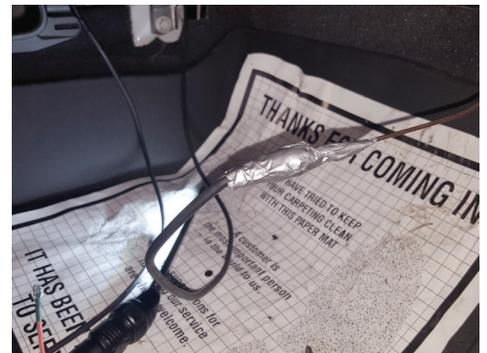
17. Cover connection with lubricant then pull hanger wire back through firewall into engine bay.
