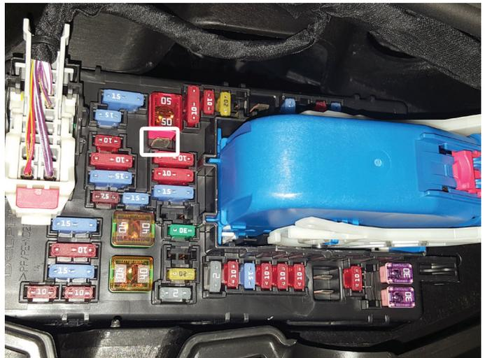
21. Connect female quick disconnect end of controller kit to fuse box.
