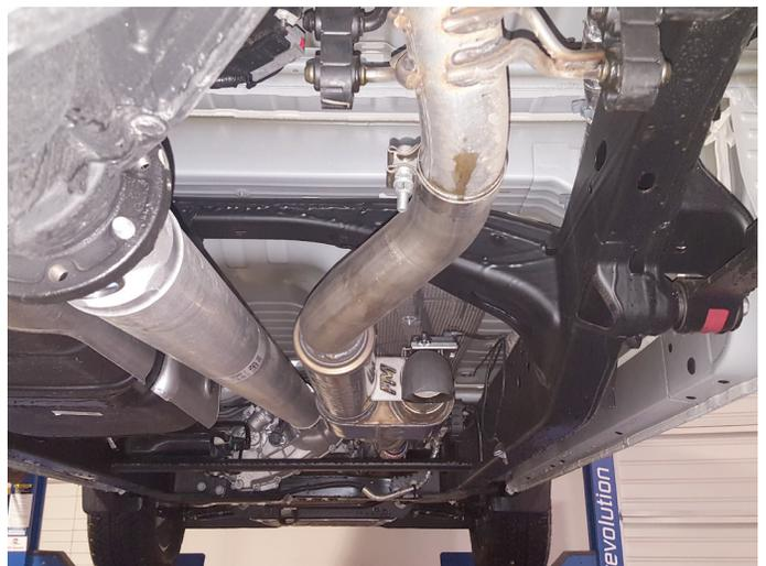
24. Adjust exhaust components for fit; maintaining ½" clearance and compensating for suspension, travel and vibration. Finally, tighten all clamps.
