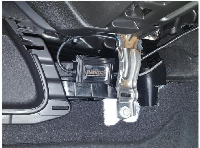
19. Remove wire, tape and lubricant from controller kit. Thread wire end down and connect it to wire assembly. Secure any slack away from moving and heated engine components.
