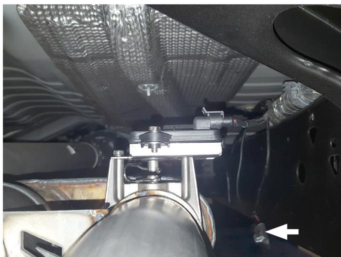
**NOTE:** You may secure wire assembly several different ways; **zip tie (12)** it to factory wire bundle, tuck it behind heat shield, secure it to frame, etc. Just be sure that connections are stable and wire is protected from heat.
