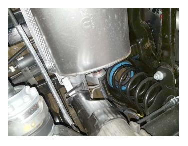
4. Support muffler and disassemble wire hangers from isolators. Loosen ball clamp, disconnect inlet pipe at cat. converter and remove exhaust system.
