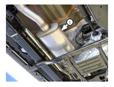
8. Place clamp (5) onto mid pipe assembly (2) then connect it to muffler. Insert wire hanger into isolators and tighten clamp just enough to allow for later adjustment.
