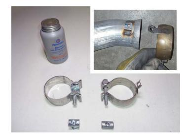
www.flowmastermufflers.com Technical Support (866) 464-6553 7. Place factory ball clamp (removed step 5) onto **muffler assembly (1)** then connect it to cat. converter. Tighten clamp enough to allow for adjustment.
