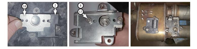
8. Place valve spring (3) into groove in muffler outlet then fasten actuator motor (4) onto mount ensuring valve spring lines up properly. Secure parts using (x3) bolt assemblies (8).
