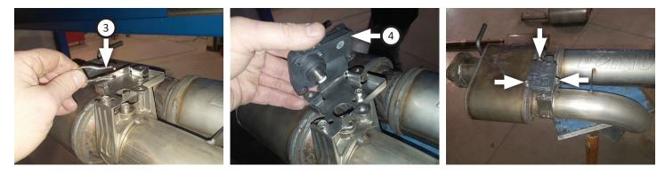
www.flowmastermufflers.com Technical Support (866) 464-6553  Fasten muffler flange to factory flange using (x2) bolts
