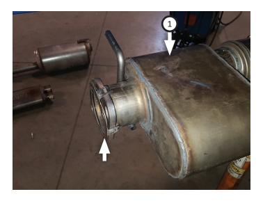
Place fiber spacer (18) onto actuator mount assembly (2), then fasten them onto muffler with (x2 ea.) fiber washers (17) and bolt assemblies (8).
