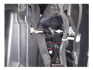
www.flowmastermufflers.com Technical Support (866) 464-6553 15. Remove wire, tape and lubricant from controller kit end. Pull wire assembly up and connect ends together. Secure any slack away from moving and heated engine components.
