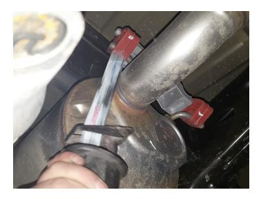
4. Remove grounding wire from hanger and bolts (x2) securing muffler flange. Remove muffler section from vehicle and disassemble flange gasket. Retain gasket for later use.
