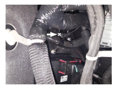
Thread hanger wire into cab through accessory point from last step. Then bend wire and connect it to controller kit end. Tape over connection to secure it.
