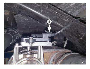
**NOTE:** You may secure wire assembly several different ways; **zip tie (14)** it to factory wire bundle, tuck it behind heat shield, secure it to frame, etc. Just be sure that connections are stable and wire is protected from heat.
