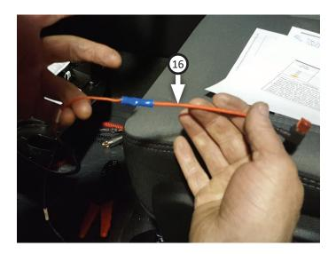
18. Pull factory fuse from F66 (Run - Accessory Feed) in fuse box. Plug it and **fuse (15)** into fused circuit tap, route wire over to fuse box then plug it back into F66 as shown. Secure any wire slack up and out of the way.
