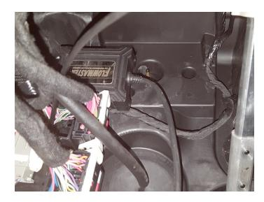
Strip end of controller kit red wire. Connect fused circuit tap (16) to it then crimp connection.
