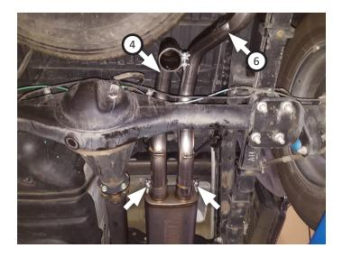
Secure left rear hanger assembly (8) to vehicle using bolt (13) through frame, mount, lock washer (14) and nut (12). Fit rubber hanger (11) onto end of hanger. Leave assembly loose to allow for adjustment.
