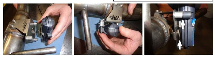
**NOTE:** Offset outlet pipe should be oriented to passenger side during install.
