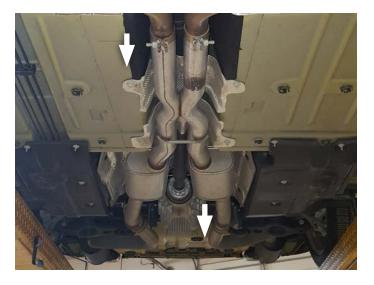
5. Remove nuts (x3) securing actuator to mounts on tailpipes. Then remove actuator and spring from mount on each tailpipe.
