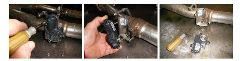
Locate factory exhaust mounts (x2) just forward of rear differential. Remove bolt securing hanger to frame, then lift hanger slightly to clear locating slot and rotate it 180 degrees. Lower hanger back into locating slot then install bolt.
