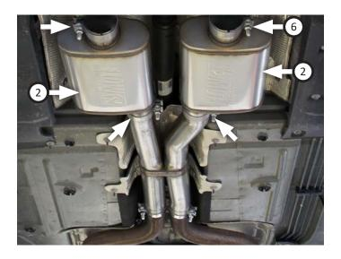
13. Transfer hangers from step 3 onto right and left tailpipes (3, 4). Connect them to mufflers, insert wire hangers (x2) into rubber isolators then rebolt rear hanger mounts to frame. Adjust tailpipes so their tips are level and centered in bumper cut-outs and tighten clamps just enough to allow for adjustment.
