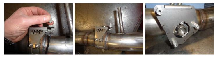
www.flowmastermufflers.com Technical Support (866) 464-6553  Insert screws (x3) (10) through actuator and flat washers (x3) (11). Place actuator onto tailpipe valve mount then tighten screws to fasten assembly. Complete step for both tailpipe assemblies. **CAUTION:** Make sure you place flat washer between actuator and standoff as shown, **NOT** beside screw head. Also, make sure the actuator spring is properly aligned between actuator and valve.
