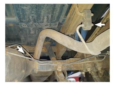
4. Support muffler and remove nuts (x2) from inlet pipe flange. Disassemble wire hangers from isolators and remove exhaust system. Retain nuts for later use.
