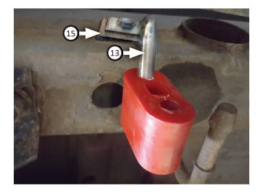
13. Route **right tailpipes (3)** and **left front (4)** over axle then connect them to muffler. Insert wire hanger into rubber hanger then tighten clamps just enough to allow for adjustment.
