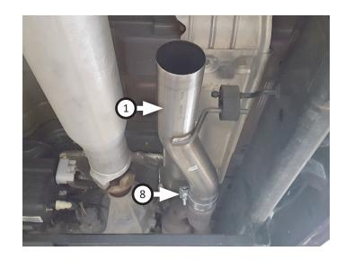
9. Place clamp (8) onto extension pipe (2 or 3) then connect it to inlet pipe. Connect wire hanger to isolator then tighten clamp just enough to allow for adjustment.
