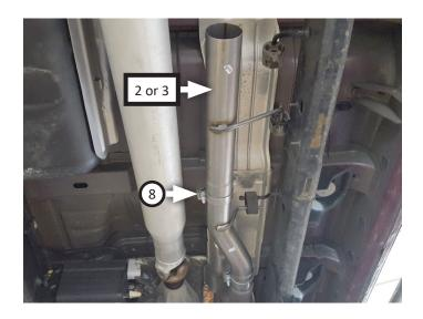
10. Place (x2) **clamps (8)** onto **muffler (4)** then connect it to extension pipe. Tighten front clamp just enough to allow for adjustment.
