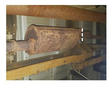
4. Separate wire hangers from isolators behind muffler. Remove bolt and hanger connecting stock tailpipe to vehicle frame. Remove tailpipe section from vehicle.
