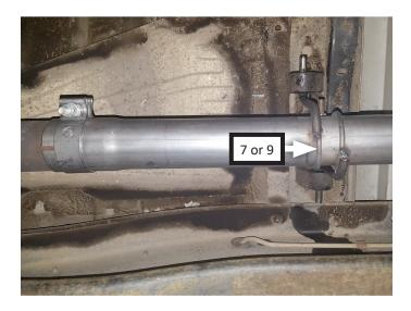
11. Place clamp (12) onto adapter pipe (1) then connect it to extension or factory exhaust. Tighten clamp just enough to allow for later adjustment.
