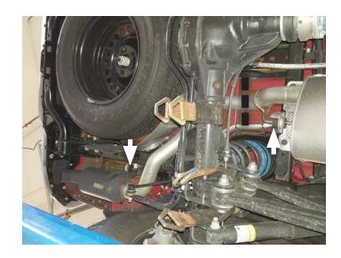
4. Loosen ball clamp from resonator inlet. Remove remaining hanger mount from vehicle frame then with help, remove resonator section from vehicle. Retain clamp and mount for later use.
