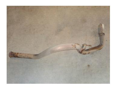
4. Measure and cut both factory muffler inlets 3" in front of their hangers. Dismount wire hangers from mounts and remove factory muffler from vehicle.
