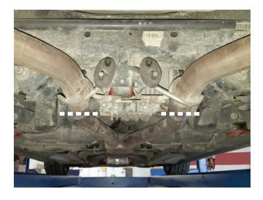
4. Support muffler then remove it from front rubber hanger mounts. Slide muffler forward to disengage and remove it. Remove and retain rear rubber mounts. Repeat procedure for remaining muffler.
