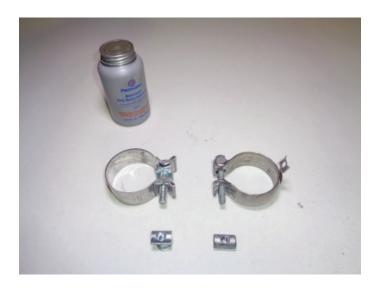
7. Place clamp (10) onto Z-notched end of inlet pipe (1) then seat it up to mark on cut factory front pipe. Orient bend as shown then tighten clamp just enough to hold.
