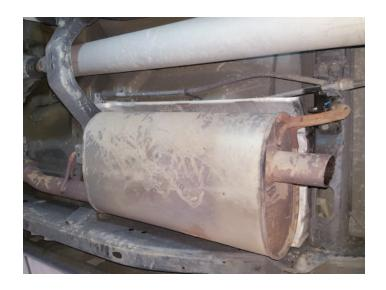
4. Support muffler then cut inlet pipe 2½" in front of muffler face. Slide muffler toward rear to disengage hanger and remove it from vehicle. Mark line 2" in front of cut inlet pipe for later exhaust install.
