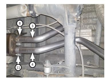
12. Place clamp (11) onto left rear tailpipe (5) then connect it to left front tailpipe. Insert wire hanger into rubber hanger then tighten clamp just enough to allow for later adjustment.
