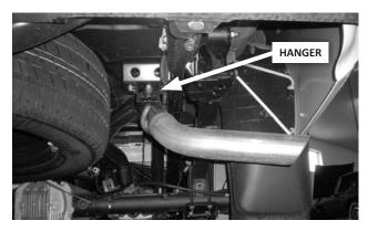
**3. Slide the tailpipe backwards** to remove it from the muffler, then move it forward to remove it from the rubber hanger.
