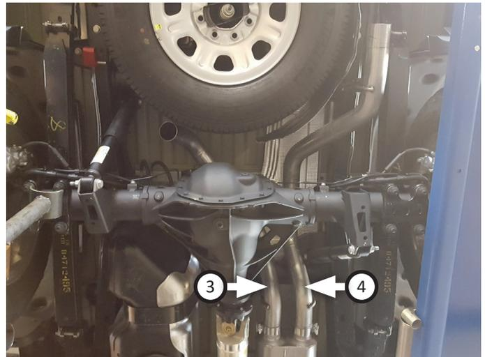
12. Place **clamp (9)** onto **left rear tailpipe (5)** then connect it to left front tailpipe. Insert wire hanger into rubber hanger then tighten clamp just enough to allow for later adjustment.
