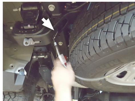
10. Fasten **left frame hanger (8)** to vehicle using **screw (14)**, **backing plate (12)**, **flat washer (15)**, **lock washer (16)** and **nut (17)** as shown. Then hang **rubber hanger (11)** on frame hanger end.
