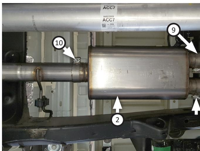
9. Some vehicles may come equipped with a spare tire clip wire. If so, remove it from its clip in point and move it inboard on vehicle frame as shown.
