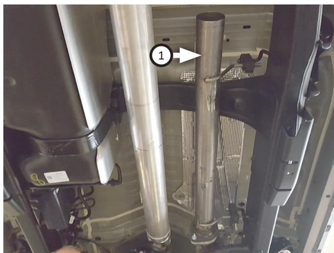
8. Place **clamp (10)** onto **muffler (2)** then connect it to inlet pipe. Tighten clamp just enough to allow for adjustment then place (x2) **clamps (9)** onto muffler outlets.
