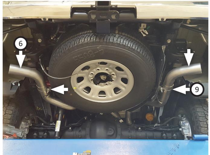
14. Place (x2) **tips (7)** onto exit pipes and tighten inlets. Rotate exit pipes and tips to desired distance from body or bumper, so angle cut on tips are properly positioned.
