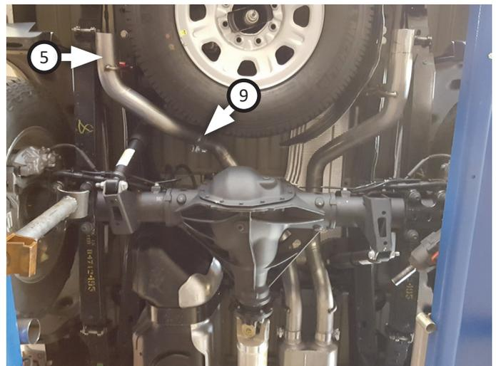
13. Place (x2 ea.) **clamps (9)** onto **side exit pipes (6)** then connect them to tailpipes and tighten clamps just enough to allow for later adjustment.
