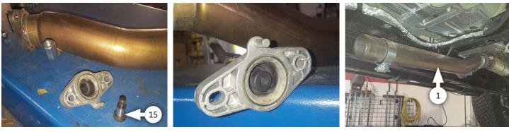
7. Place clamp (6) onto the mid pipe (2), situate the pipe over the axle, and connect it to the inlet pipe. Snug the clamp just enough to allow adjustment during system assembly.
