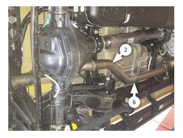
Fasten the right hanger (4) to the passenger-side frame studs with 2 lock nuts (14). Fasten the left hanger (5) to driver-side frame using 2 bolts (8) and flat washers (10) inside the frame, and 2 lock washers (11) and nuts (9) against the hanger. Install the 2 rubber hangers (7) on the hanger rods.
