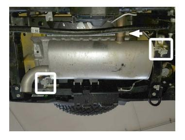
4. Support the front pipe, then remove the flange fasteners. Unbolt the isolator mount from frame, separate rear wire hanger from isolator, then remove front pipe from vehicle.
