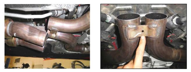
5) Carefully deburr the ends of the front pipes where cut with a file or die grinder. The next step will be to remove the brace between the two front pipes.
