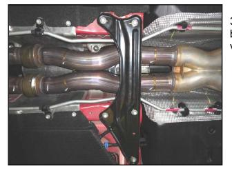
3) Using a 13mm socket or wrench, remove the five bolts securing the body brace to the bottom of the vehicle.
