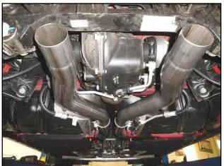
2) Place a provided 3.00" clamp onto the slip-fit of mid pipe **#26614S** and slide onto the back of the left side Scavenger outlet. Connect the hanger on the pipe to the rubber mount on the vehicle and tighten the clamp enough to hold in place. Repeat this step on the right side of the vehicle with mid pipe **#26615S**. You can now follow the installation section of the instructions provided with your new Flowmaster axle-back system.
