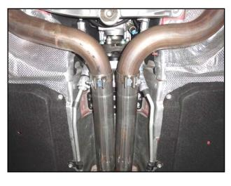
1) Place a supplied 2 <sup>3</sup>/<sub>4</sub>" clamp onto the inlets of Scavenger assembly **26611S**, place the assembly onto the front inlet pipes and slide on approximately 3.00". Be sure the Flowmaster embossing in the center of the assembly is facing the ground. Re-install the body brace and tighten securely.
