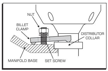
Figure 1 Correct Billet Hold Down Installation.
