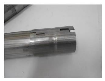
1) Slide the supplied **TB809S** adapter pipes onto the end of each outlet of the **86341S** X-pipe assembly. Place a supplied clamp onto the connections and tighten enough to hold.
