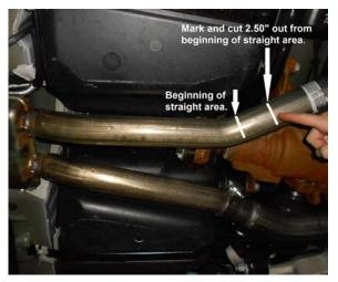
2) Begin by measuring back 2 ½" from the beginning of the straight area shown in the photo at left and make a mark on both pipes. Support the exhaust system both in front and behind the area to be cut. Check that the marks are correct, then using a sawsall, cut both pipes at the marks. **Note: Due to the closeness of the pipes to the gas tank, use caution when cutting!** Carefully deburr the end of the muffler inlet pipes where cut with a file or die grinder.
