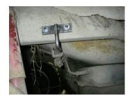
On the frame, in the rear wheel well, there are two  $\frac{1}{4}$ " threaded holes in the frame on either side of the vehicle. This is where hanger **#425HA** will be mounted on both sides of the vehicle to support the rear of the tailpipes. Use the  $\frac{1}{4}$ " x 1" bolts, washers and lock washers to secure the two hangers into place. Then slide the **#HA168** rubber hanger onto the two hangers. If these holes are not threaded, see the helpful hints on page 4 for instructions.
