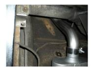
4) On the underside of the vehicle slightly forward of the rear axle there are a pair of holes on either side of the vehicle that will be used to mount the rear muffler hangers, #424HA (left side) and #423HA (right side). Once mounted, the two hangers will point toward the center of the vehicle.
