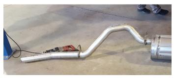
4. Remove studs (x2) from catalytic converter flange on factory exhaust. You will be using different fasteners to install your new Flowmaster exhaust system.
