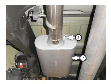
10. Place rear clamp hanger (4) onto muffler outlet and hang it in isolators. Route tailpipe assembly (3) over rear axle and connect it to muffler, insert wire hanger then tighten clamp hanger for later adjustment.
