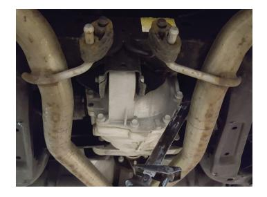
5. Detach wire hangers from isolators then remove (x2) tailpipes from vehicle.
