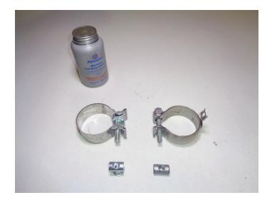
7. Place (x2) clamps (4) onto left (1) and right (2) mufflers then connect them to factory pipes and mount wire hangers in isolators. Tighten clamps just enough to allow for adjustment.
