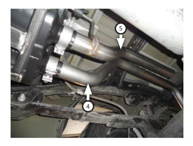
11. Place clamp (10) onto left rear tailpipe (6) and connect it to left front tailpipe. Insert wire hanger into rubber hanger and tighten clamps just enough to hold parts.
