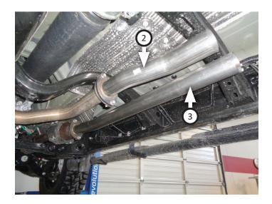
8. Place left (11) and right (12) inlet pipe clamp hangers onto inlet pipes and hang them on vehicle frame hanger mounts. Place (x2) clamps (10) onto muffler (1) then connect it to inlet pipes. Tighten clamps enough to allow for adjustment.
