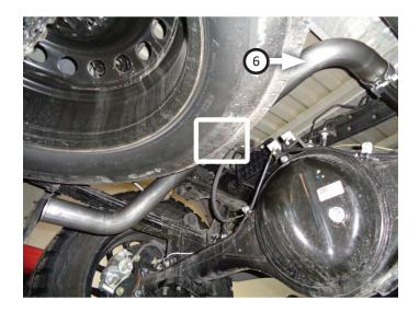
**NOTE:** This kit includes both side and rear exit pipes. If you wish to equip your vehicle with a rear exit exhaust, use rear exit pipes now in place of side exit pipes.
