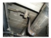
Place a provided 21/2" clamp onto the muffler outlet and then place tailpipe 6) #16770S into position over the rear axle. Slide the hangers on the pipe into the rubber mounts on the vehicle and then into the muffler outlet. Tighten the clamp enough to hold, but still allow adjustment.
