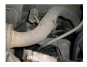
Using a hacksaw or sawsall, cut the stock tailpipe off where it exits the 2) muffler. (This step is not mandatory, but it makes removal a little easier.)
