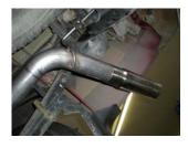
7) Place stainless tip **#ST429** onto the end of the tailpipe and adjust the tip to the desired position. Tighten the nut on the tip to hold securely in place.
