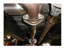
2) Place the inlet pipe onto the back of the existing OEM head pipe and fasten using the nuts, bolts and washers provided in the hardware kit. Tighten just enough to hold in place, but still allow for adjustment. The S-shaped pipe will be offset toward the frame of the vehicle.
