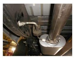
4) Place the inlet of muffler #8530570-262 thru the #382HA clamp hanger and onto the inlet pipe, support with a stand. Level the muffler and tighten the clamp just enough to hold in position, while still allowing for adjustment.
