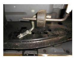
3) Slide clamp hanger #382HA over the back of the inlet pipe and insert the hanger into the factory rubber mount bolted to the side of the frame. Do not tighten this clamp yet. If the extension pipe is used, use the provided 3" band clamp at the connection between the inlet and extension pipe. Note: If the 382HA hanger doesn't line up with the rubber mount, the mount may need to be re-located slightly forward and down to the other set of factory mounting holes in the frame.
