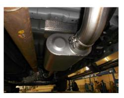
5) Slide a 3.50" clamp onto the muffler outlet neck. Place tailpipe #36047S into position over the axle and insert the hanger at the front and rear of the pipe into the rubber mounts on the vehicle and slide into the muffler outlet. Tighten the clamp just enough to hold, while still allowing for adjustment.
