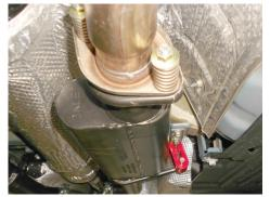
11. Place clamp (6) onto right muffler (4) then connect it to y-pipe outlet. Insert wire hangers into rubber hangers then tighten clamp enough to hold parts.
