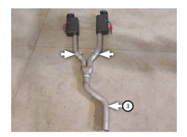
9. Set stands in place under vehicle to hold y-pipe assembly in place then set Y-pipe on stands.
