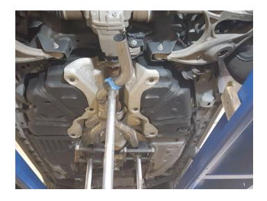
Secure Y-pipe in place by securing hangers with bolts (removed step 5). Then connect flanges with (x2 ea.) steel spacers (8), bolts (7), flat washers (11) and springs (removed step 4).
