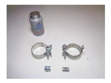
8. Place (x2 ea.) rubber hangers (9) and front frame hangers (5) onto left (2) and right (1) resonators. Place (x2) clamps (6) onto Y-pipe (3) then connect resonators to it. Tighten clamps just enough to connect parts.
