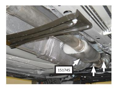
Place clamp (MC225BS) on intermediate pipe (16738S) and connect it to resonator assembly. Insert wire hanger into isolator and tighten clamp just enough to allow for adjustment.
