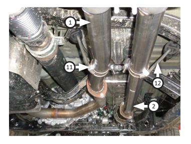
8. Place (x2) **clamps (10)** onto **muffler (3)** inlets then connect it to inlet pipes. Tighten clamps just enough to allow for adjustment. Then place (x2) **clamps (10)** onto muffler outlets.
