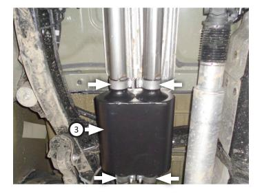
Connect right (4) and left front (5) tailpipes to muffler outlets. Place clamp (10) onto left front tailpipe then connect left rear tailpipe (6) to it, routing it over axle. Insert wire hangers into isolators then tighten all clamps enough to allow for adjustment.
