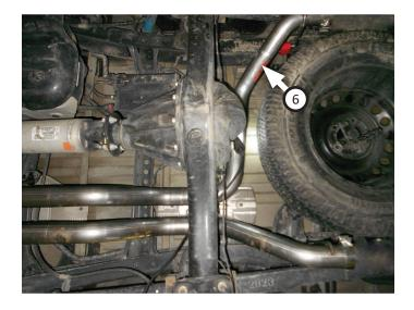
**NOTE:** This kit includes both side and rear exit pipes. A side exit is preferable for towing purposes, to avoid blowing fumes in or on vehicles you may be towing (eg: RV trailer, boat, etc). Otherwise, complete this step using **rear exit pipes (7)** in place of side exit pipes.
