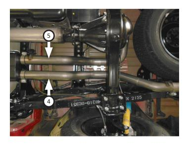
10. Locate large hole in square cavity on left rear frame rail. Install backing plate (15) on top side of frame and left rear hanger (14) below, using flat washers (x2) (18), lock washer (19) and nut (17) to fasten it. Finally, slide rubber hanger (16) onto hanger rod.
