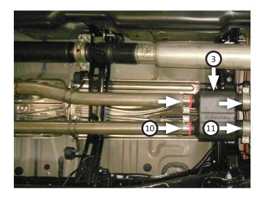
9. Connect **right and left front tailpipes (4, 5)** to muffler outlets. Tighten clamps just enough to allow for adjustment.
