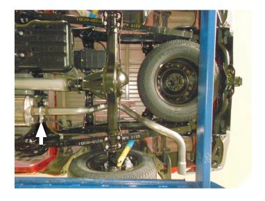
4. Remove bolts (x4) from front flange connections.
