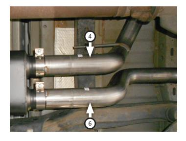
13. Place clamp (13) onto left rear tailpipe (5) then connect it to left front tailpipe. Insert wire hanger into rubber hanger then tighten clamp just enough to allow for later adjustment.
