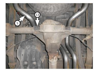
14. Place (x2 ea.) clamps (13) onto side exit pipes (7) then connect them to tailpipes and tighten clamps just enough to allow for later adjustment.
