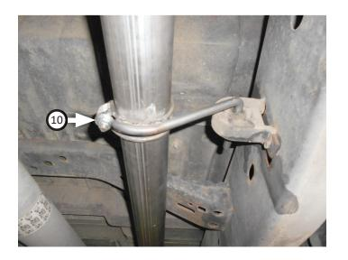
10. Place clamp (13) onto muffler (3) then connect it to inlet or extension pipe. Tighten clamp just enough to allow for adjustment then place (x2) clamps (13) onto muffler outlets.
