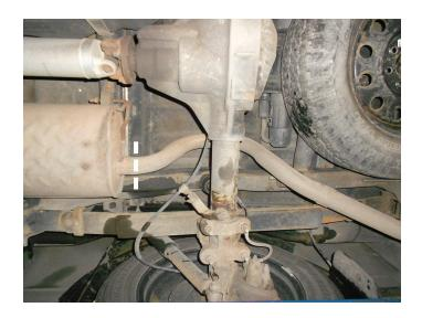
4. Support muffler and disassemble wire hangers from isolators. Loosen clamp, disconnect inlet pipe at catalytic converter and remove exhaust system.
