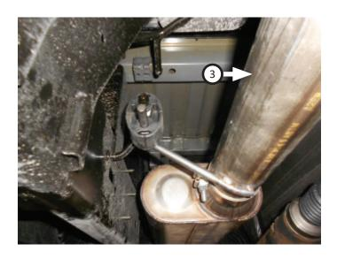
Place clamp (14) onto muffler (4) inlet then connect it to extension pipe. Tighten clamp just enough to allow for adjustment then place clamps (x2) (15) onto muffler outlets.
