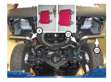
17. Recommended: apply one inch tack weld to all slip-fit connections then apply high temperature paint over each weld to prevent rust and premature corrosion.
