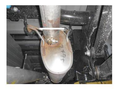
4. Support muffler and remove all hangers from isolators on muffler assembly; then remove clamp on slip connection just behind catalytic converter. Heat or cut to separate connection and remove muffler assembly.
