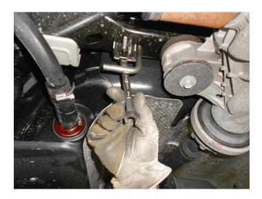
Place a clamp (7) onto inlet of each Super 44 muffler
