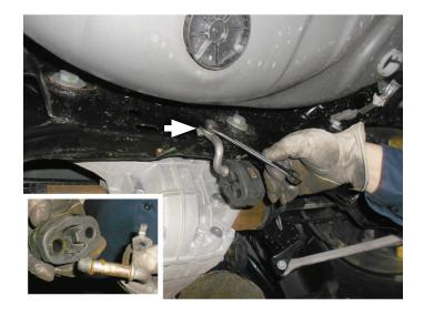
8. Install **left tailpipe hanger (5)** with bolt and washer (removed step 7) to front of mount beside rear differential on drivers side of vehicle oriented as shown. Place rubber isolator onto hanger.
