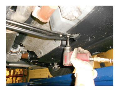
4. Support muffler and disassemble wire hangers from isolators. Un-clip ground strap from middle hanger on right tailpipe. Loosen clamps behind catalytic converters and with help, lower and slide system back off from head pipes and set it carefully on ground.
