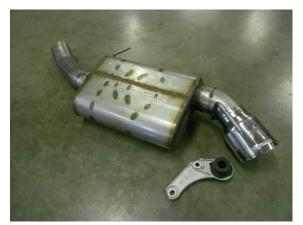
1) Place the new Flowmaster muffler units next to the factory unit and swap the rear hanger mounts from the stock muffler to the Flowmaster assemblies.
