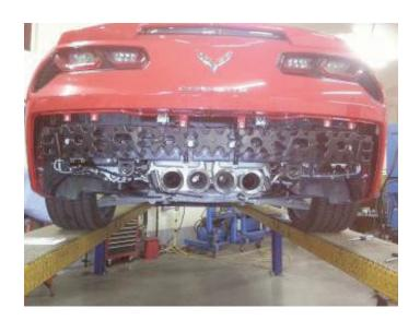
Find clamp connection on each pipe just forward of rear sub-frame and axles. Loosen nut on each clamp.
