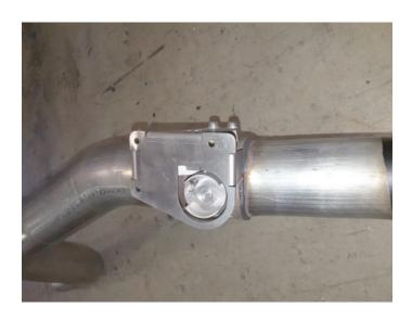
12. Route each muffler up and over axle into clamped connection. Secure hanger mounts to frame using fasteners (removed step 9).
