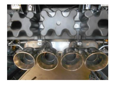
**NOTE:** The GM service manual recommends conducting an **ACTUATOR LEARN PROCEDURE** on this exhaust system once changed. Should your vehicle throw a check engine light or malfunction, find a GM dealer to complete said procedure.
