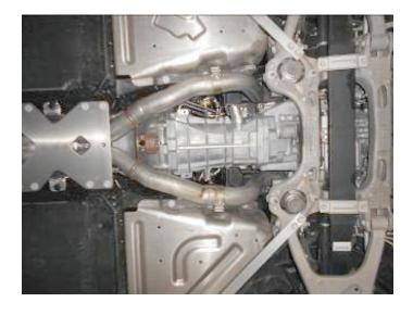
9. Disassemble both muffler assemblies by unbolting their hanger mounts, loosening front connection then pulling them out over axle. Transfer hanger mounts from factory to Outlaw mufflers and retain bolts for later.
