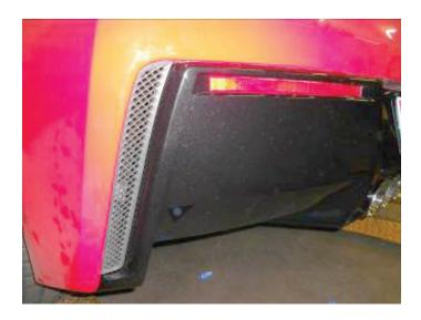
5. On each side of bumper fascia is a thin horizontal red reflector held in place with clips. Use a small flat blade screw driver to very carefully pop out reflectors. Then remove hex bolts (x4) securing fascia to bumper frame and under license plate location.
