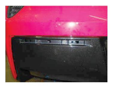
6. Remove hex bolts (x2) in cavity just above exhaust tips. With assistance, remove panel secured along top edge with clips. Grasp panel at one end through vertical slot, carefully pull it out and set it aside.
