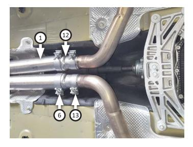
10. Place (x2) clamps (5) onto scavenger pipe (1) inlets then slide it 2" onto stock head pipes (offset outlet pipe should be oriented to passenger side). Level and center assembly in drive line tunnel then tighten clamps just enough to hold parts.
