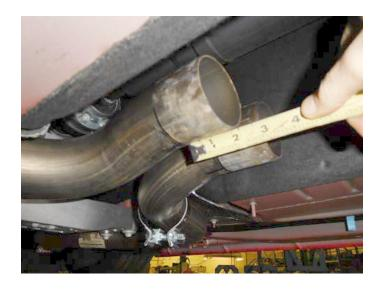
11. Place (x2) clamps (6) onto both muffler (4) inlets then connect them to scavenger pipe, sliding them 1¾" deep. Level mufflers and tighten clamps just enough to hold parts but still allow for adjustment.
