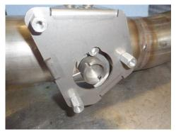
8. Place (x3) screws (10) into actuator and through (x3) flat washers (11). Fasten assembly to mount on tailpipe, aligning actuator spring into slot on mount before tightening fasteners. Repeat step on remaining tailpipe.
