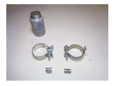
Apply threadlock to fasteners then thread (x3) screws
