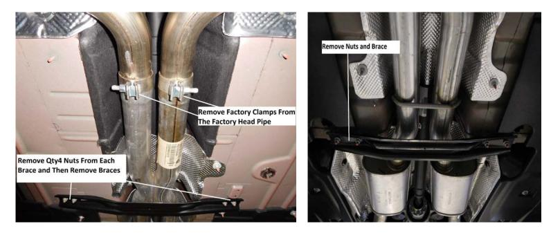
3) Place a stand under the rear of each tailpipe to support the rear of the system. Just forward of the rear differential, you will find two exhaust valve actuators, one mounted to the side of each tailpipe. Carefully unplug the wire from the actuator and tuck away for reconnection later.
