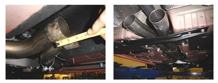
4) Place a supplied 3" clamp onto the inlet neck of both mufflers. Slide the mufflers onto the back of the Scavenger pipe assembly about 1-3/4" and support with stands. Level the mufflers and tighten the clamps enough to hold, but still allow for adjustment.
