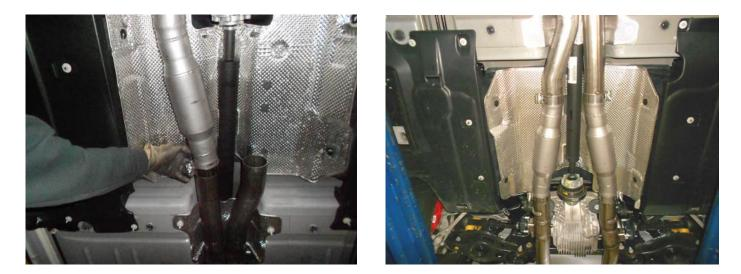
5) Place a supplied clamp onto the left muffler outlet. Place the left tailpipe **# 26654S** into position and starting from the rear, connect the hangers on the tailpipe to the rubber mounts on the vehicle. Slide the tailpipe fully into the muffler outlet and adjust the tailpipe so that the end of the pipe is centered in the factory exhaust bezel. See photo below. Tighten clamp enough to hold, but still allow for adjustment. Repeat this step for right tailpipe **# 26652S**.
