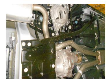
4. For vehicles equipped with heat shields; remove them by cutting through their rear straps, then lift and lower them a few times to break remaining weld.
