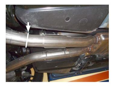
**NOTE:** Use caution as you cut pipes to avoid cutting other engine components.
