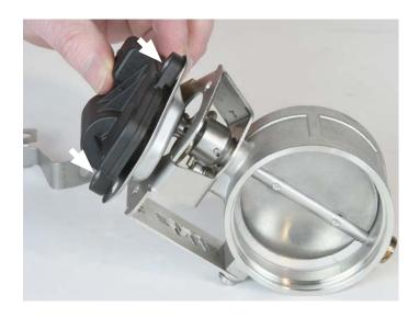
13. Place each wire loom bracket onto left and right actuator (as indexed from step 10) then fasten assemblies exactly as shown (x3 ea.) screws (5), spacers (4), split lock washers (6) and hex nuts (7).
