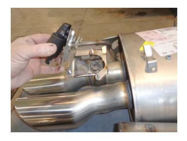
12. Install actuator onto valve by lining spring arm to valve shaft notch then lower it into place. Rotate actuator assembly holes to line up with mount holes.
