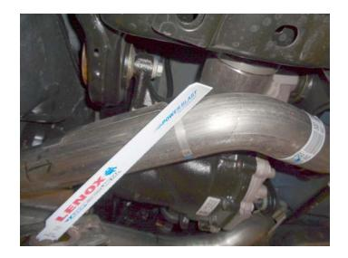
5. Mark each pipe just behind second bend (where bend straightens out). Then, at rear of each muffler, unplug wire to actuator and tuck connection away until later.
