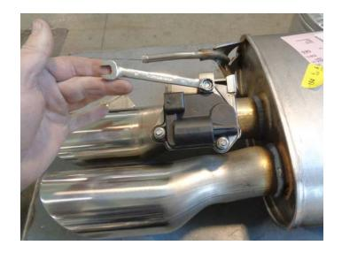
11. Lift actuator with heatshield and spring attached from factory valve assembly.
