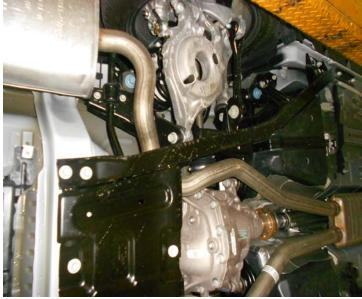
2) On convertible model vehicles, the body braces shown in the photos above will need to be removed in order to remove the factory system and install the Flowmaster system. Starting at the front of the right side (passenger) brace, loosen the front bolt and then work your way to the rear of the vehicle removing the next eight bolts, lower the brace from the vehicle. Repeat this step on the left side of the vehicle with the six bolts on that side.
