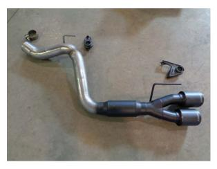
1) Place the new Flowmaster muffler units next to the factory units and swap the front and rear hanger mounts from the stock mufflers to the Flowmaster assemblies. Also, place a provided 2-1/2" clamp onto the inlet of each assembly. Tighten the clamp just enough to hold in place.
