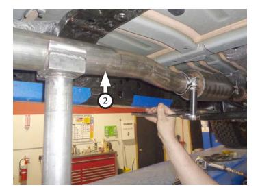
10. Place **clamp (5)** onto **over-axle pipe (3)**, route it over and into inlet pipe. Insert wire hanger into isolator on vehicle then tighten clamp just enough to allow for adjustment.
