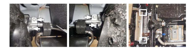
4. Loosen clamp at muffler inlet connection above rear axle then remove muffler from vehicle.
