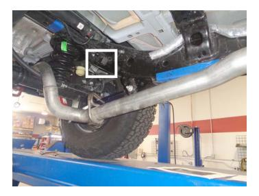
7. Loosen clamp at resonator inlet and remove resonator assembly from vehicle. Retain clamp for later re-use.
