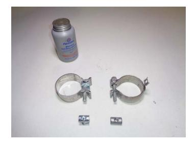
9. Place clamp (3) onto right muffler assembly (1) then connect it to cut pipe and support it. Re-install rear and front hanger mounts to frame. Repeat step with left muffler assembly (2) on left side of vehicle.
