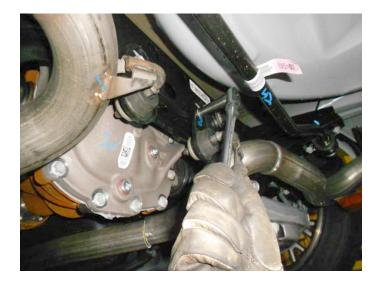
6. Carefully deburr factory pipes at cut ends. Remove hanger mounts at rear of vehicle from vehicle frame then transfer all mounts from factory system to corresponding side on Flowmaster system.
