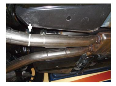
6. Mark both pipes 5" back from straight portion in previous step. Verify measurements then cut pipes at each mark. Unbolt hangers then remove muffler assembly and deburr pipes.
