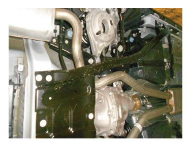
4. Remove (x2) heat shields by cutting through strap at rear, then lifting and lowering shield a few times to break weld.
