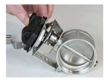
www.flowmastermufflers.com Technical Support (866) 464-6553  Place each wire loom bracket onto left and right actuator (as indexed from step 10) then fasten assemblies exactly as shown (x3 ea.) screws (5), spacers (4), split lock washers (6) and hex nuts (7).
