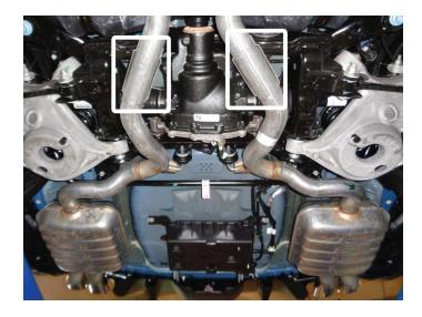
5. Make mark just past second bend of each pipe, where bend ends and straight area begins. At rear of each muffler, unplug wire to factory exhaust actuator then tuck connection out of the way.
